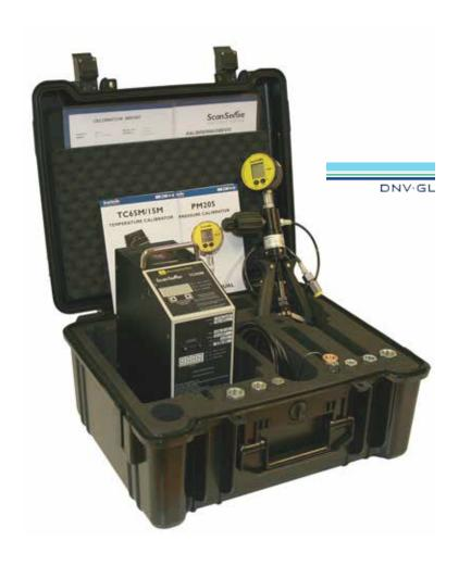
Our Mini test Case meet most applications on board Mercantile Vessels as well as Naval Vessels and mobile Offshore Drilling Units refer to pressure and temperature. Our Mini system makes it easy to adjust to the specific needs you might have on certain vessels for pressure and temperature. All Test Cases comes complete with necessary accessories.
